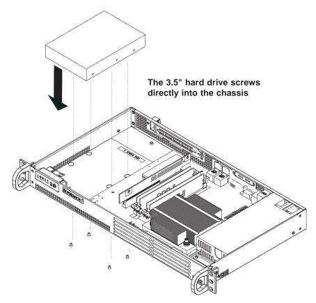
Figure 6-3. Installing a 3.5" Hard Drive
